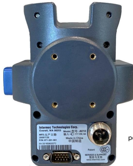
Note: Vehicle Dock must have external power connected for USB port to be active.
